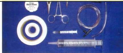
Tools needed to check and repair the glider pneumatic system.
