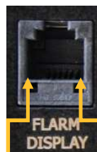
FLARM DISPLAY 1 2 3 4 5 6 Pin numbers
