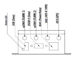
PowerFLARM Core has the following connectors:
