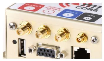
A-version devices (part No. FLAPFCnnA and FLAPFDnnA): FLARM A and B ports are reverse polarity female SMA connectors with a pin as center conductor. ADS-B is a standard female SMA connector with a female center sleeve.
