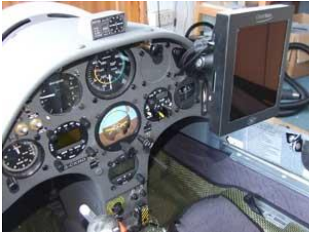
RAM Mount Kit used to mount a ClearNav to the instrument panel
